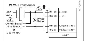
4 to 20 mA control signal for Non-Spring Return and **Electronic Fail-Safe**
